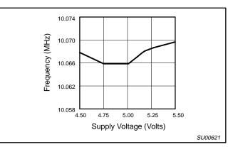
Figure 5. Supply Voltage vs. Frequency
