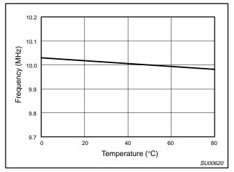
Figure 4. Frequency Variation Using N750 Capacitors
