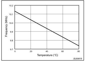
Figure 3. Frequency Variation Using NPO Capacitors
